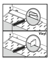
$\sqrt{\phantom{a}}$  Put spacers between the planks and the wall when installing your floor. They provide a uniform and sufficient expansion joint of 8 to 10 mm/0.32 to 0.39in.. Place the spacers about every 30 cm/ 1 ft.
